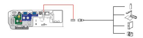
If you connect a digital camera, USB flash drive, or USB storage device, you can use the projector's Slideshow feature to project images. See the online User's Guide for details.
